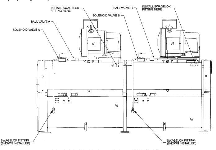
Fig. 2 — Installing Fittings and Valves, 30HX (Typical)
